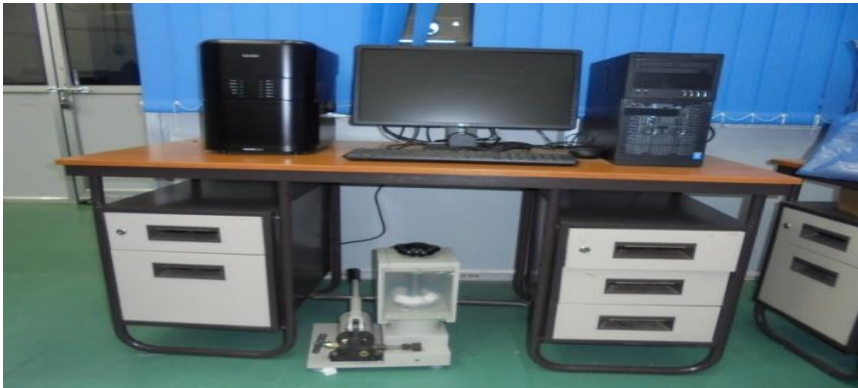
Precision Multiferroic Test System ( P-E , piezoelectric, piezoelectric, magneto-electric for bulk and thin-films) with temperature variation facility (Make: USA Radiant Technologies Inc., USA)
